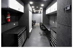
MISSION // The U.S. Air Force required a mobile solution for responding to crashed, damaged, or disabled aircraft incidents on or off airfield property. Response needs dictated a durable trailer with a climate-controlled work area, mobile power, and secure storage for power tools and other equipment.
