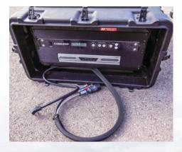
The one button auto acquisition controller locates and precisely aligns the antenna in all three axes to the required satellite.
